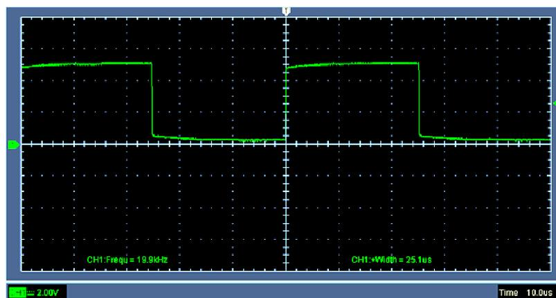
Fig. 8. Generator signal at the ATmega328 microcontroller PD0 output, Oscillogram
