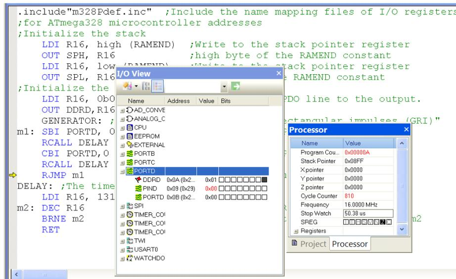
Fig. 7. GENERATOR program debugging window in AVR Studio
