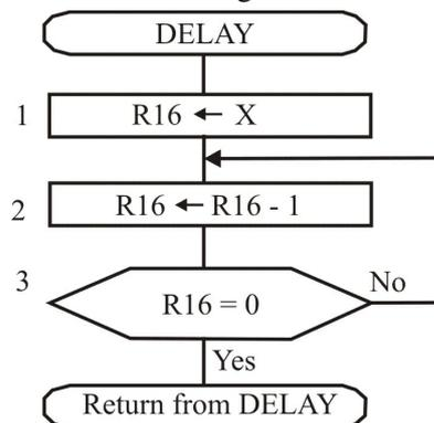
Fig. 2. Algorithm of the DELAY subroutine
