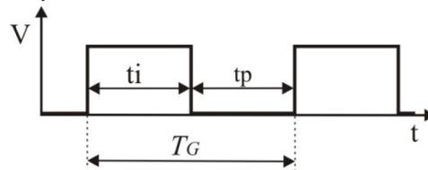
Fig. 1. Generator signal, Timing Diagram
